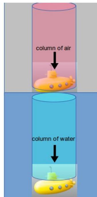
Illustration 1: Columns of fluid above the submarine.
