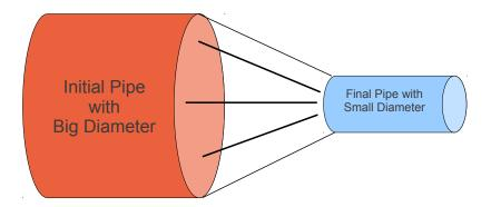
Volume Flow Rate<sub>1</sub> = Volume Flow Rate<sub>2</sub>  $A_1v_1 = A_2v_2$
