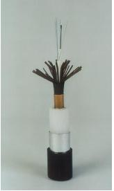
Illustration 5: Fiber optic cable is protected on the outside by several layers of material.
