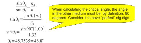
This is the critical angle for water to air.
