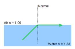
Illustration 3: The incident angle is so big that the refracted ray never truly leaves the water.
