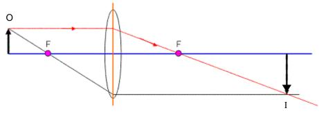
*Illustration 3: Rule 2 is parallel to the principle axis.*
