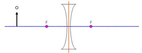
Illustration 5: A diverging lens with an object on the left hand side.
