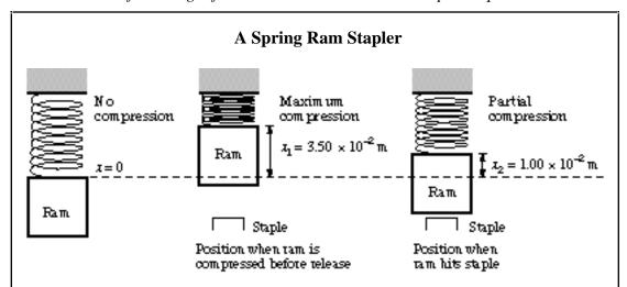
Heavy-duty stapling guns use powerful springs in combination with a small metal rod (called a ram) to produce the impact necessary to move staples or nails into materials such as wood, wallboard, or even concrete.
