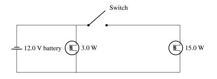
• Describe what happens to the 3.0 W bulb and the 15.0 W bulb when the switch is open and when it is closed in the two-light-bulb circuit.
