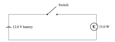
• Draw and label a second schematic diagram containing one switch, the 12.0 V battery, and a 3.0 W nightlight bulb in parallel with the 15.0 W bulb. Design this two-light-bulb circuit so that the switch controls only the 15.0 W bulb.
