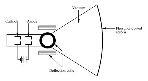
Electrons are "boiled off" the surface of the cathode and are accelerated toward the anode. The cathode is  $4.5 \, \text{cm}$  from the anode. A potential difference of  $2.5 \times 10^3 \, \text{V}$  exists between the cathode and the anode. The electrons are deflected both side to side and up and down by pairs of magnetic deflection coils mounted on the neck of the tube.
