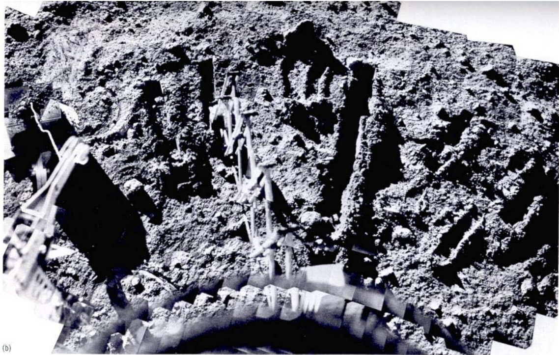
FIGURE 7-33.—(a) Early view of surface-sampler operations area showing bearing strength test sites, a , and object, b , which was selected for magnetic-attraction test on the basis of its luster, shape, and gray tone. (b) Surface-sampler operations area after trenching efforts (Catalog 7-SE-16).
